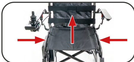
Illustration 12. Folding the frame.
