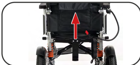
Illustration 11. Folding the frame.
