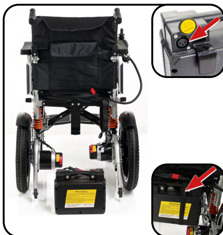
Illustration 14. Disconnecting the battery and charging outside the wheelchair.
