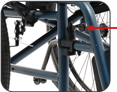
Illustration 5. Footrest locking lever. Push to unlock the footrest.
