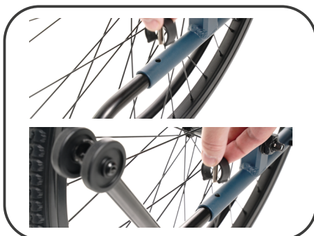
Illustration 13. Rotation of the anti-tip wheels.
