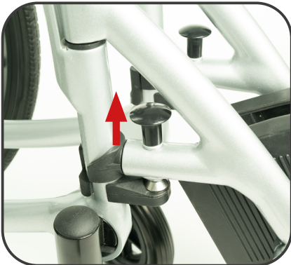
Illustration 5. Footrest lock. Pull upward to unlock the footrest rotation.
