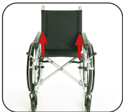
Illustration 9. Folding the wheelchair.
